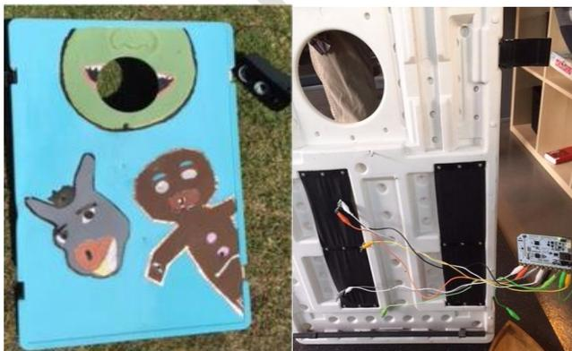
**Figure 4. Front and back of Bean Bag Stand, painted with conductive ink and connected to Touchboard microprocessor.**
